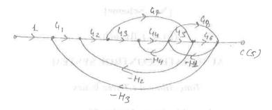
(d) Obtain C(s)/R(s) of the system shown in fig. using block diagram reduction rule:
